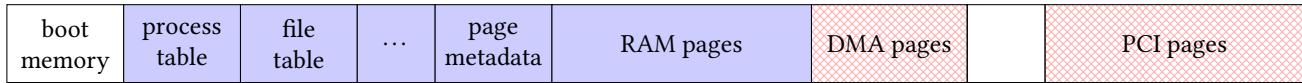
Figure 6: Memory layout in Hyperkernel: boot memory is used only during kernel initialization; shaded regions are accessible only by the CPU; and crosshatched regions are accessible by both the CPU and I/O devices.
