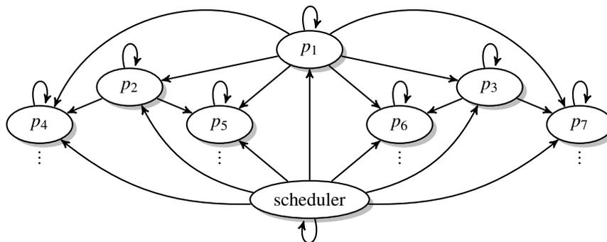
Figure 2: The isolation policy of NiKOS+. Each process can have up to two child processes in this case.
